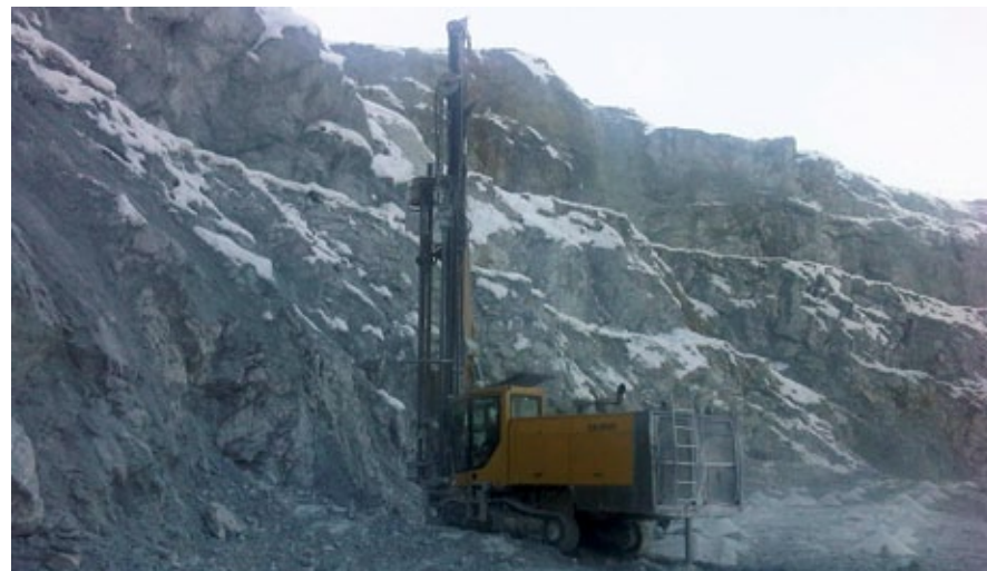
Eti Bakır Murgul copper mine is owned by Cengiz İnşaat using ROC L8 drill rigs at their open-pit copper mine. They are drilling with Atlas Copco Down the hole hammer 165 mm.
